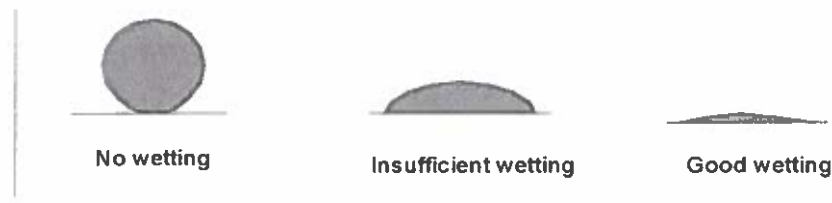
Figure 5-6. Schematic representation of wetting a surface by a liquid.
