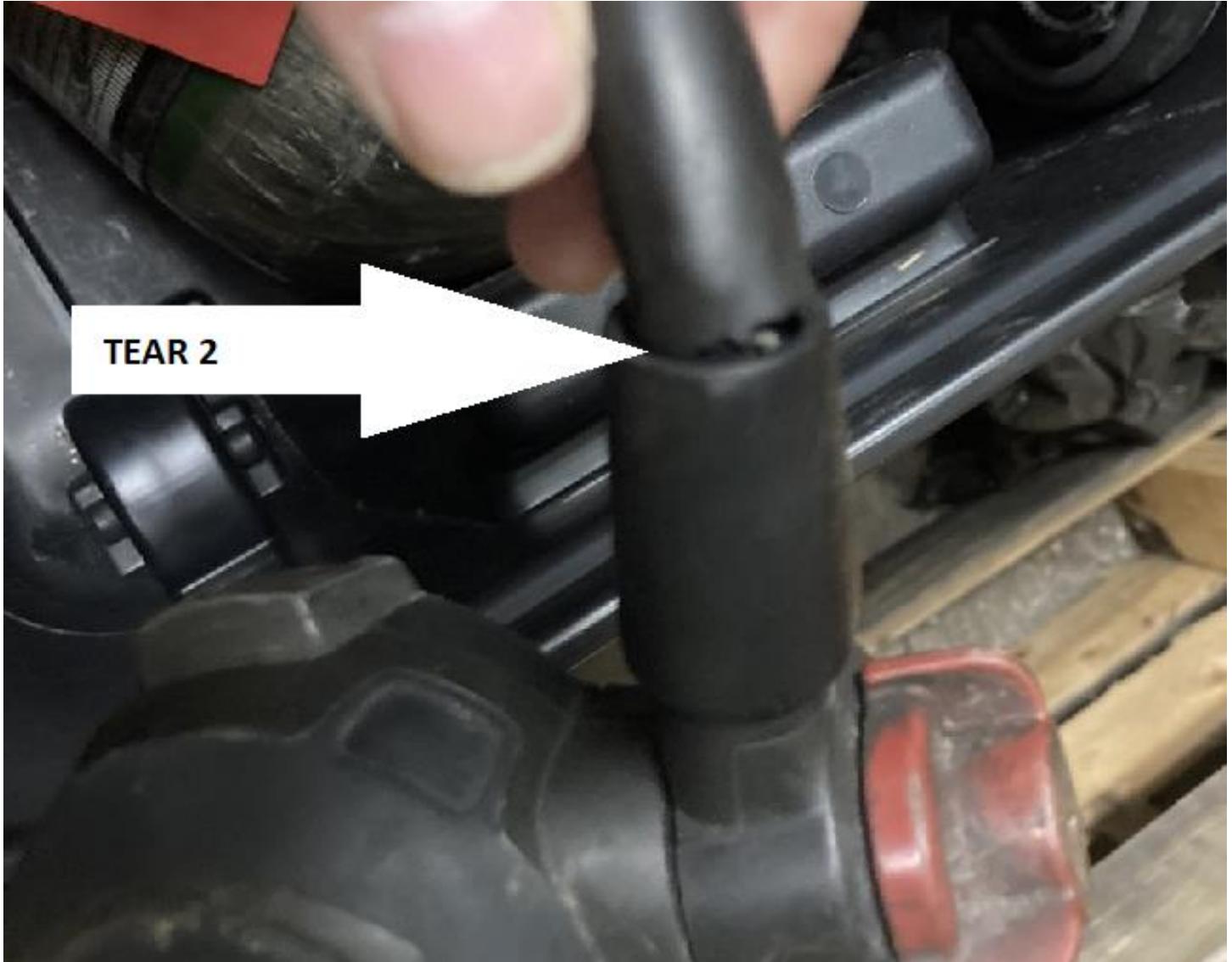
Figure 7 - Tear 2 close-up (photo credit: affected department)
