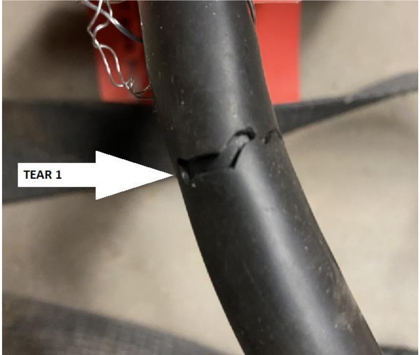
Figure 6 - Tear 1 close-up (photo credit: affected department)
